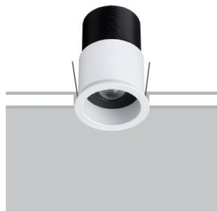
The Jimbo range of recessed fixtures offers adjustable optics in which, by working on an adjustment element, it is possible to change the opening of the light beam from 10° to 55°, in order to adapt to the project needs.
