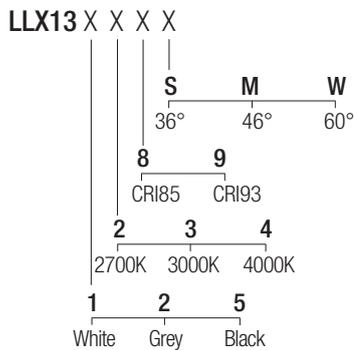
**Note:** The finishing refers to the outer ring of the luminaire only, the inner part of the optical compartment is always black.
